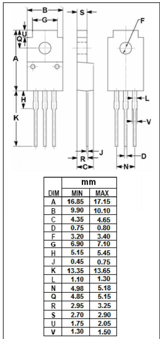
**isc Silicon PNP Darlington Power Transistor****2SB1342****ELECTRICAL CHARACTERISTICS**T<sub>j</sub>=25°C unless otherwise specified
