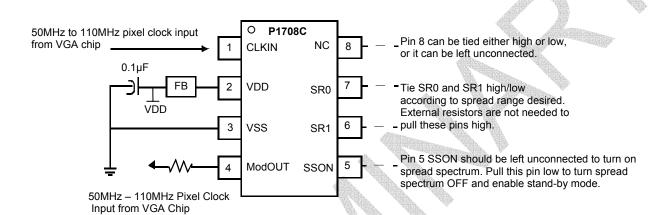
Note: To set the P1708C to standby mode, disable the input clock (pin 1 CLKIN) and pull SSON (pin 5) low. Refer Standby Mode Selection Table.
