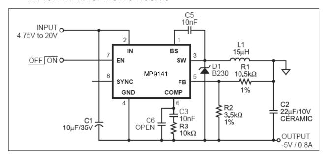
Figure 3—Application Circuit for -5V Supply
