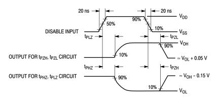
Figure 2. 3-State AC Test Circuit and Waveforms (t<sub>PLZ</sub>, t<sub>PHZ</sub>, t<sub>PZH</sub>, t<sub>PZL</sub>)
