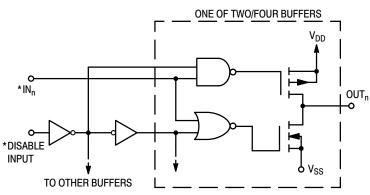
\*Diode protection on all inputs (not shown)
