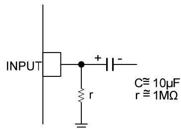
This IC requires  $0.1\mu\text{F}$  capacitor between INPUT and GND,  $1\text{M}\Omega$  resistance between INPUT and GND for clamp type input at mute mode.
