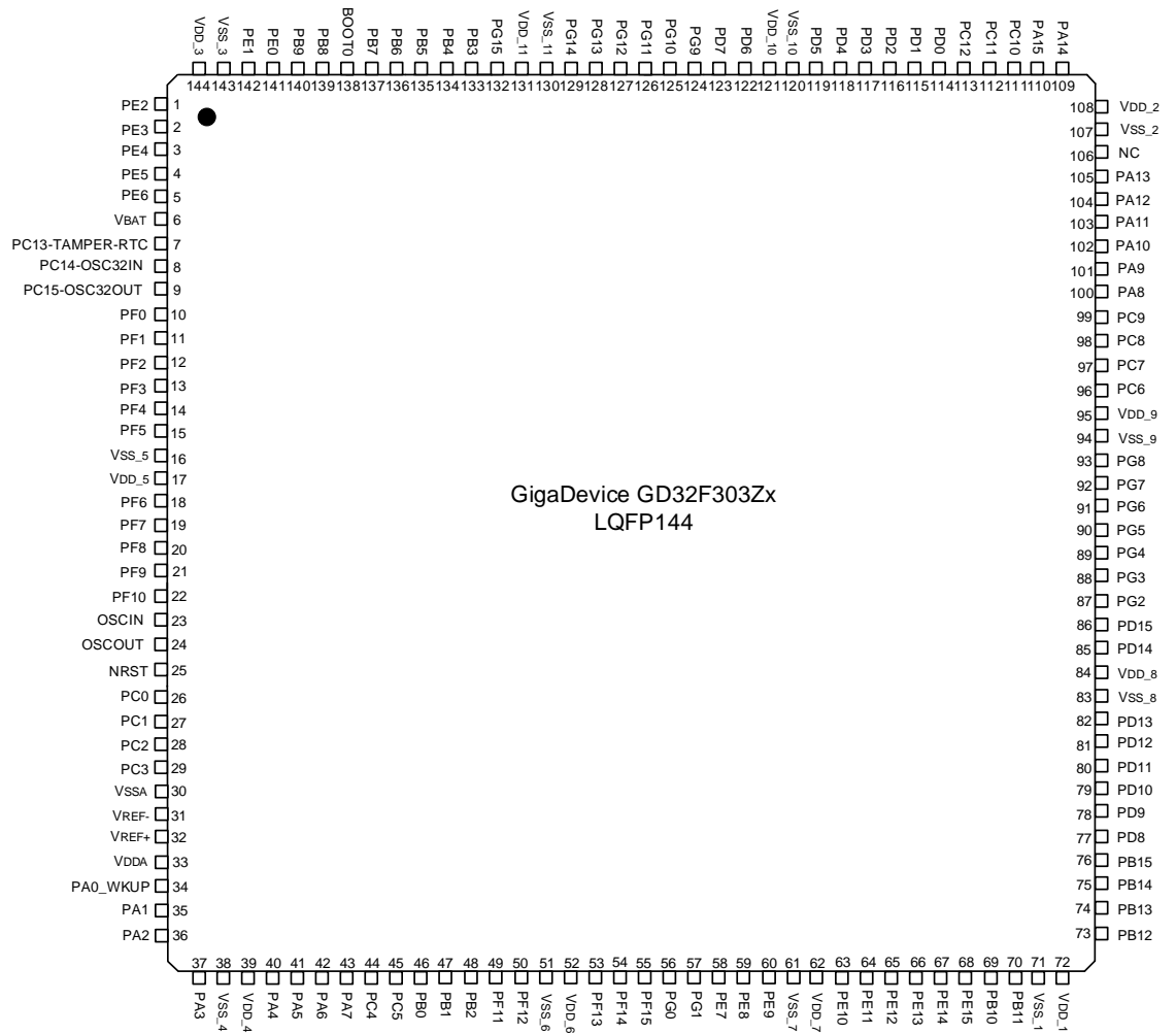
Figure 2-2. GD32F303Zx LQFP144 pinouts
