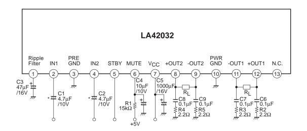
\* LA42032 employs the zero-bias type input circuit, with the input pin potential being nearly zero (about 0.01V). Accordingly, the polarity must be determined according to the DC potential of a circuit connected to the previous stage of LA42032.
