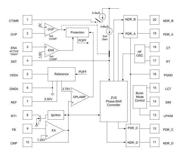
Figure 2. Functional Block Diagram
