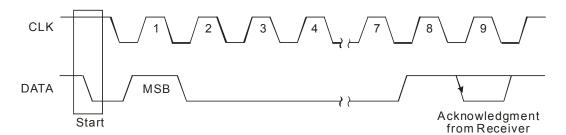
The audio processor that has been addressed has to generate an Acknowledge after receiving each byte, otherwise, the SDA Line will remain at the High Level during the ninth (9th) Clock Pulse. In this case, the master transmitter can generate the STOP Information in order to abort the transfer.
