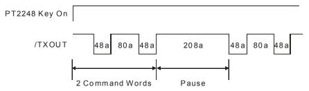
When any of the continuous keys is depressed, the above continuous signal transmits a repetitive cycle of 2 command words and then a pause (with a pause duration of 208a) until the key is released.
