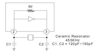
When the oscillation frequency is set at 455 KHz, the carrier wave of the transmitting signal is set at 38 KHz. Unless the keys are being operated, the oscillation is normally stopped; thereby, reducing power consumption.
