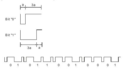
One word of the transmission command is in the configuration of (010110010001).
