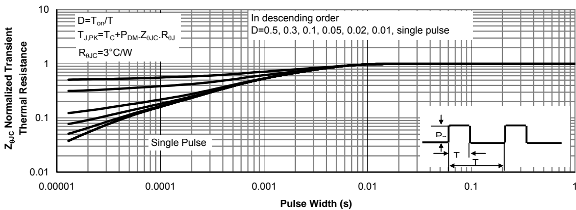
Figure 11: Normalized Maximum Transient Thermal Impedance (Note F)
